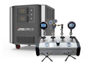
The pressure source of the SPMK213G-D electric pressure reducer calibrator uses digital control technology to generate high-stability pressure quickly. The required pressure is controlled by the precision valve on the console to meet the requirements of field and laboratory calibration works, which also can test gas pressure reducers, ordinary pressure gauges, pressure transmitters, and pressure switches.
